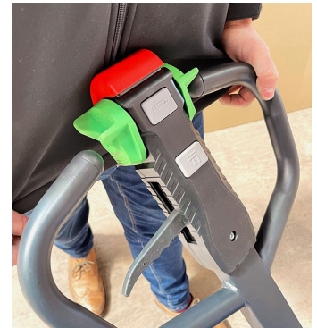
Secondary emergency stop at the top of the control handle
