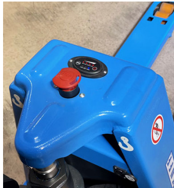
Emergency stop, on/off, battery and fault code indicator
