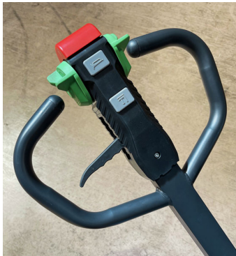
Fork lifting, lowering and drive controls
